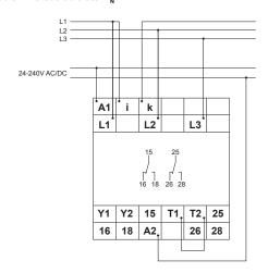
Connected 3~ with fault latch I<sub>N</sub><12A
