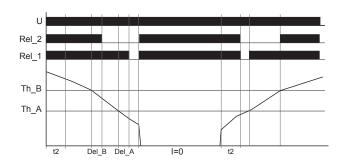
Example: I=0 Inv. with minimum monitoring (2MIN+I=0 ON) relay state invers: Rel\_1 and Rel\_2 off
