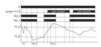
Example: Window function (WIN) - Resetting the fault latch by pressing the plus- and minus-key (+ & -)
