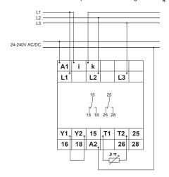
Connected 1~ without fault latch but with current transformer I,>12A
