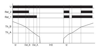
Example: I=0 with maximum monitoring (2MAX+I=0 ON) relay state normal: Rel\_1 and Rel\_2 off
