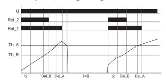
Example: I=0 Inv. with maximum monitoring (2MAX+I=0 ON) relay state invers: Rel\_1 and Rel\_2 on
