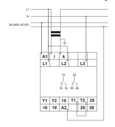
Connected 3~ with fault latch and current transformer I<sub>N</sub>>12A
