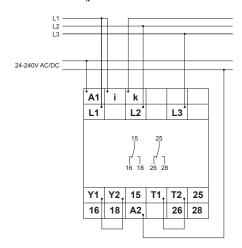
Connected 3~ with fault latch and temperature monitoring sensor I<sub>N</sub><12A
