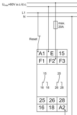
Range 300V, supply voltage 400V a.c. without fault latch
