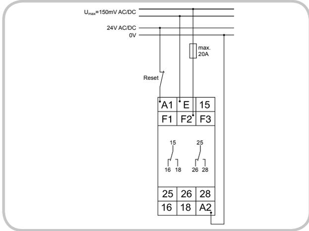
► Range 10V, supply voltage 24V AC/DC and fault latch
