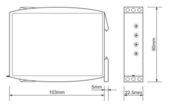
G2PM400VFA02 with power module TR2 230V a.c.
