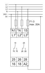
G2FW50HzYFA02-Italia 3-phase mains with switching power supply SNT2 24V DC
