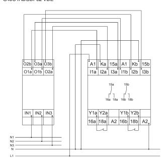
Note that the terminals A1-A1 and A2-A2 are internally connected.
