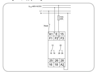
Range 300V, supply voltage 24V AC/DC and fault latch
