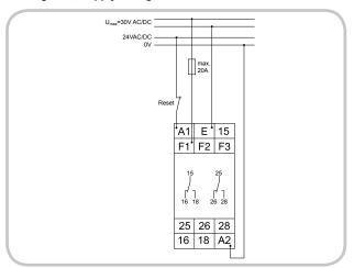
Range 60V, supply voltage 230V AC and fault latch
